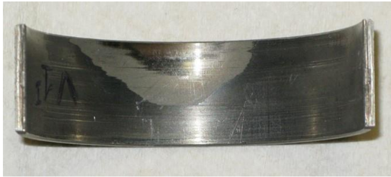
Figure 19. Edge loading on main bearing.
